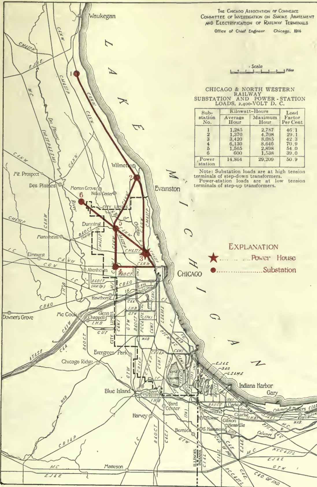
FIG. 624. LOCATIONS OF POWER STATION AND SUBSTATIONS FOR THE CHICAGO & NORTH WESTERN RAILWAY FOR THE 2,400-VOLT D. C. SYSTEM
